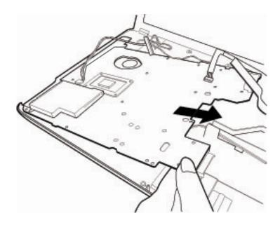
Figure 4-30 Removing Main PCB
